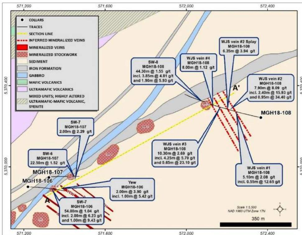
**Figure 5: Windjammer South and Gap; Drill Location and Geological Interpretation Map**
