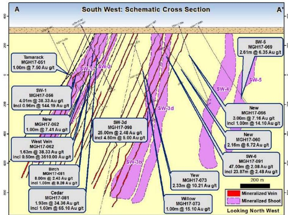
**Figure 4: South West; Schematic Cross Section (Selective results)**
