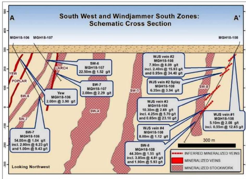
**Figure 6: Windjammer South and South West; Schematic Cross Section**
